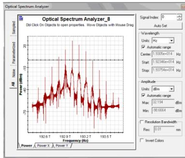
Fig 8: Spectrum analyzer at output of SOA (FWM Generation) when both inputs are high
