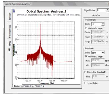
Fig 9: Spectrum analysis at the output of SOA when both inputs are zero
