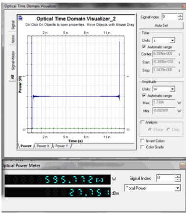
Fig 5: Time domain visualizer and optical power meter output at A=0, B=1
