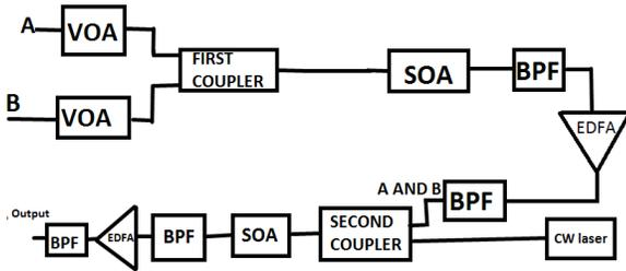
Fig 1(a) Block Diagram of optical NAND gate
