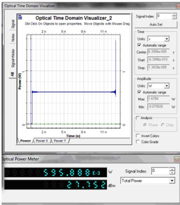
Fig 4: Time domain visualizer and optical power meter output at A=0, B=0
