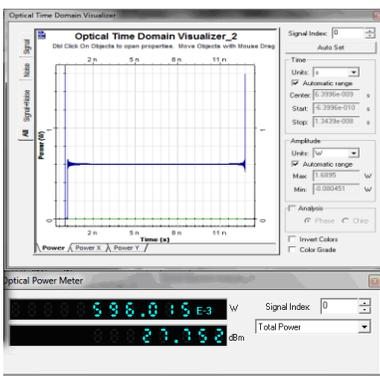
Fig 6: Time domain visualizer and optical power meter output at A=1, B=0
