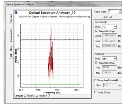
Fig 3: Spectrum analyzer at the output of second SOA when both inputs are high
