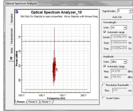
Fig 2: Spectrum analyzer at the output of second SOA when both inputs are low
