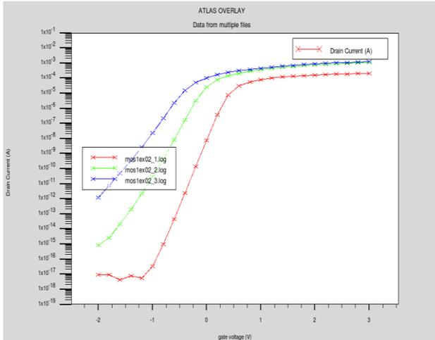
**Figure 5 Log  $I_d$ - $V_{gs}$  characteristics of 90nm MOSFET (with LDD) at different drain voltages**
