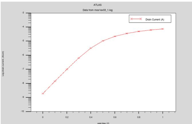
**Figure 2 Log  $I_d$ - $V_{gs}$  characteristics of 90nm MOSFET**
