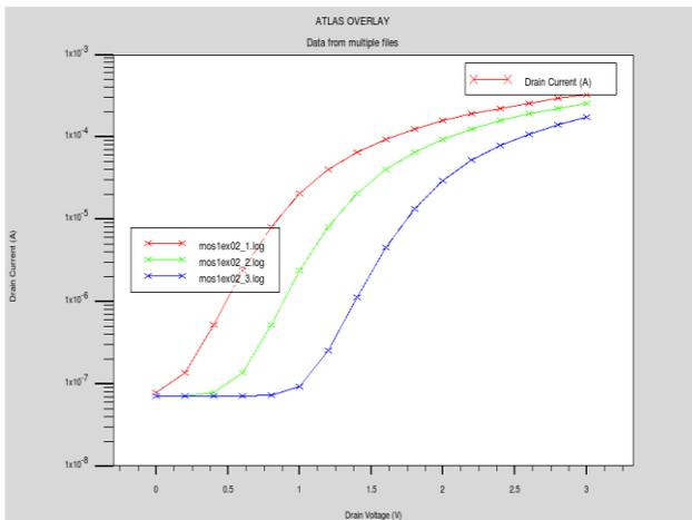
**Figure 6 Log  $I_d$ - $V_{ds}$  characteristics of 90nm MOSFET (with LDD) at different drain voltages with work-function engineering**
