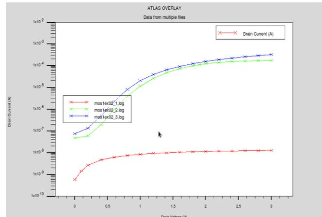
**Figure 4 Log  $I_d$ - $V_{ds}$  characteristics of 90nm MOSFET at different drain voltages**
