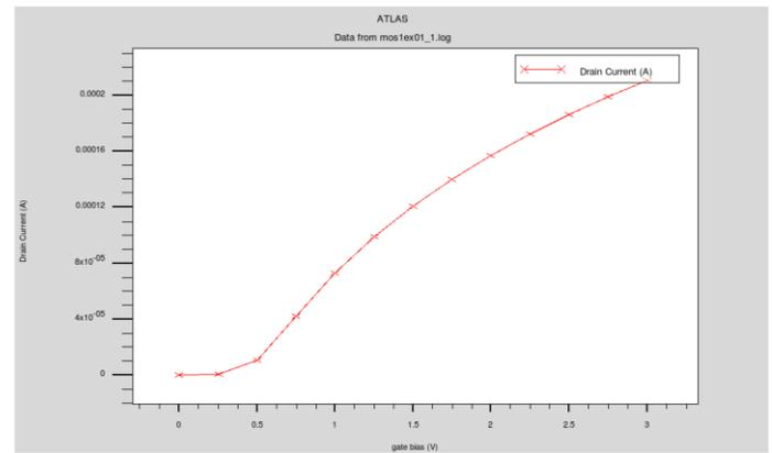
**Figure 3  $I_d - V_{gs}$  characteristic for 90nm n-channel NMOS**
