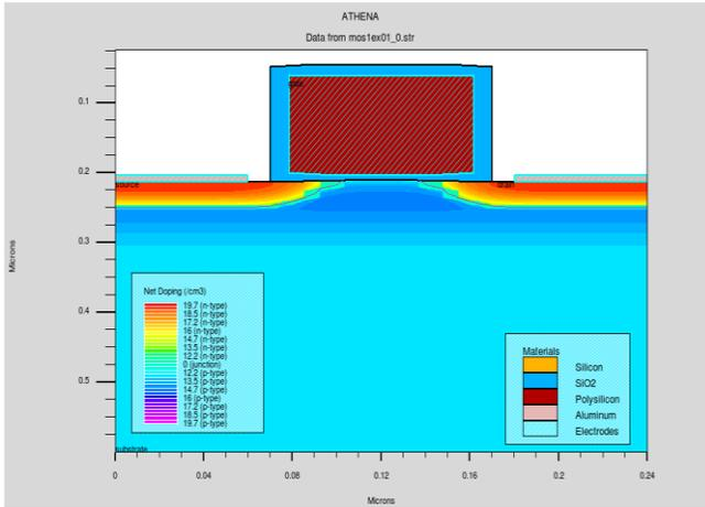
**Figure 1. Structure of 90 nm MOSFET in Athena**
