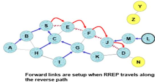
Figure 5: Forward Path Setup in MDSR AODV
