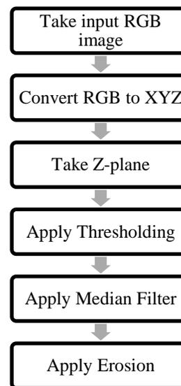
Fig. 1 Algorithm for Segmentation Using XYZ Plane
