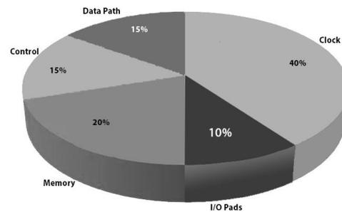
Fig. 1. Power dissipation in a typical CPU
