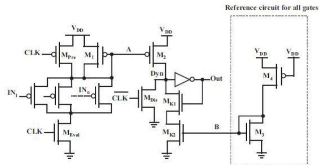
Fig. 5. The current comparison domino (CCD) for implementation of wide fan-in gates[7]
