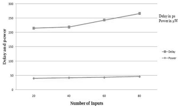
Fig. 18. Relationship between delay and power consumption of the tag comparator used CDL circuits in terms of the number of input.
