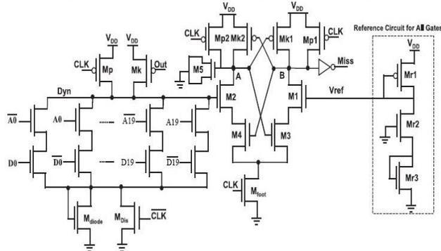
Fig. 16. The 20-bit tag comparator implemented by single version of the comparison-based dual-rail domino (CDL).
