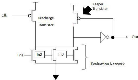
Fig. 2. Wide fan-in OR gates using the standard footless domino (SFLD).
