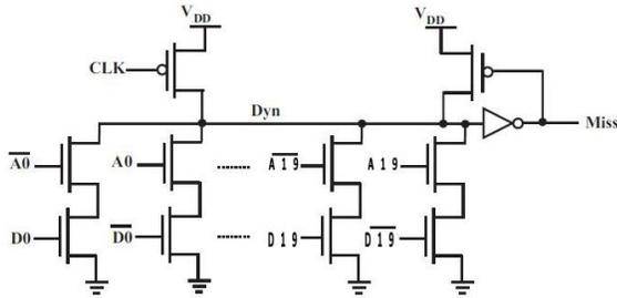
Fig. 15. The 20-bit tag comparator implemented by standard footless domino(SFLD).
