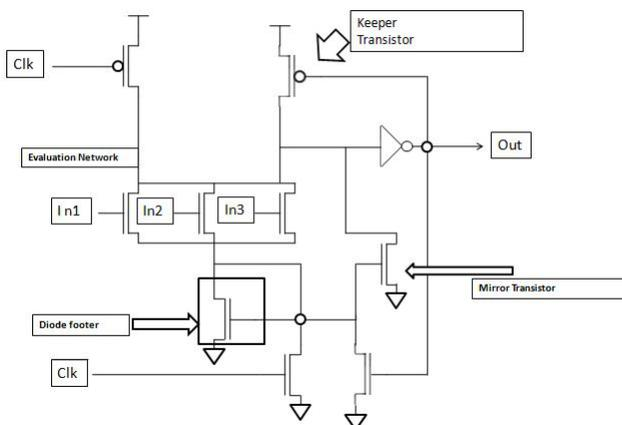
Fig. 3. Diode footer transistor configuration.
