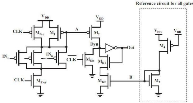
Fig. 6. The comparison-based dual-rail domino (CDL) [8].
