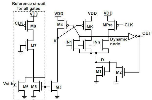
Fig. 4. The controlled keeper by current-comparison domino (CKCCD) [6]
