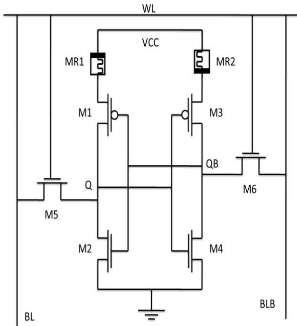
Fig.1. 6T Memristor based SRAM cell
