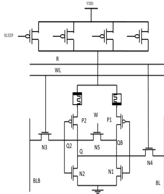
Fig.5. Sleep Technique employed 7T Memristor based SRAM
