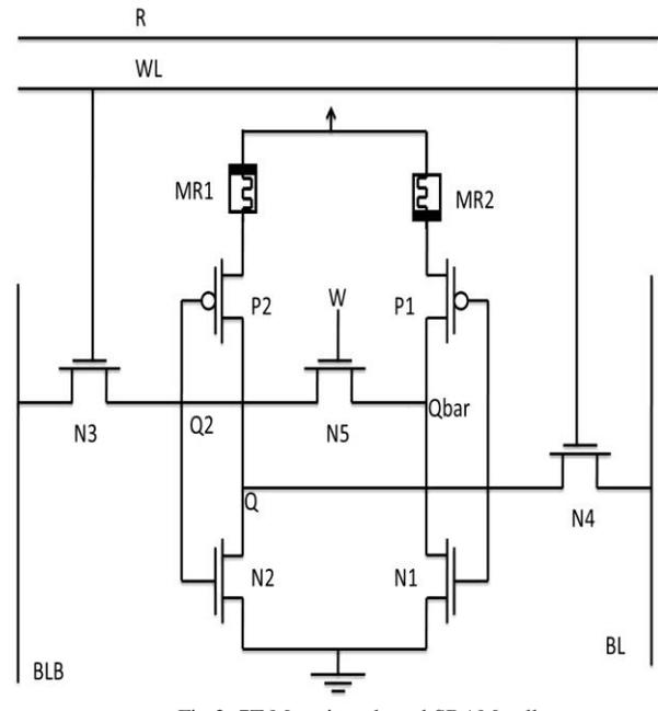
Fig.2. 7T Memristor based SRAM cell
