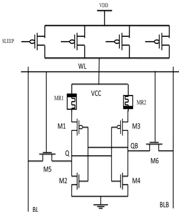
Fig.4. Sleep Technique employed 6T Memristor based SRAM
