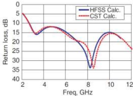
**Figure 2.** Return loss of the planar monopole eclipse antenna With  $r = 10$  mm,  $d = 6$  mm,  $S = 0.4$  mm,  $g = 0.3$  mm.
