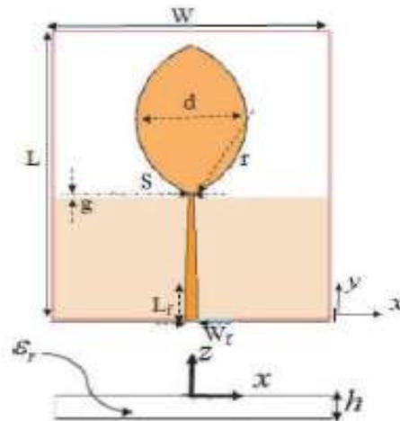
Figure (1) Proposed monopole eclipse antenna design
