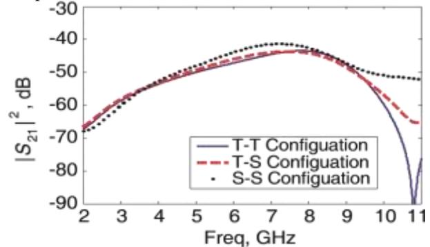
**Figure 4.** Magnitude of transfer functions of the three different configuration of the monopole eclipse antenna
