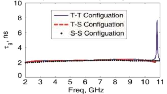
**Figure 5.** Group delays of the three different configuration of the monopole eclipse antenna
