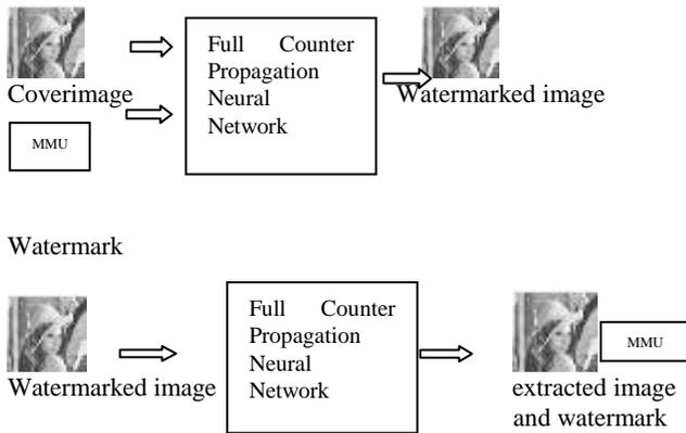
Figure 3: Schematic Block Diagram of FCNN
