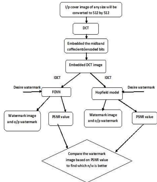
Figure 2: Flow Chart for Digital Water marking using FCNN and Hopfield Model
