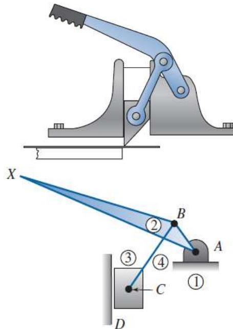
Fig. (1a): Shear Press Fig. (1b): Kinematic Diagram for shear Press
