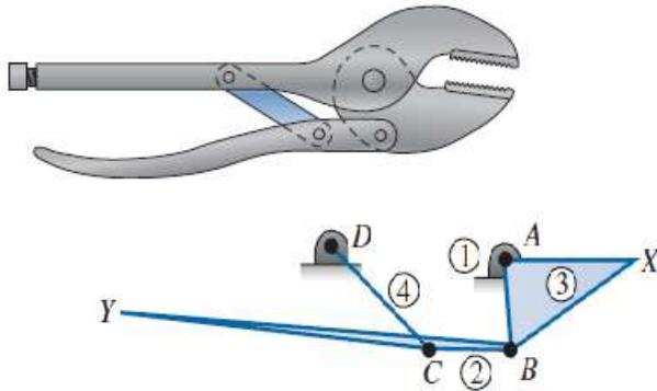
Fig. (2a): Vise Grips Fig. (2b): Kinematic Diagram for Vise Grips
