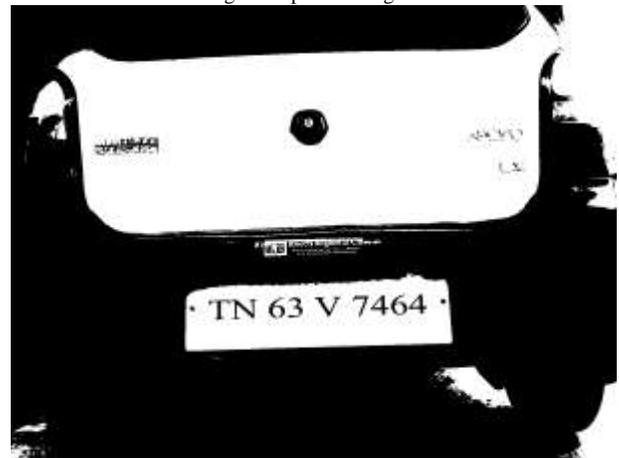
Fig. 3. Global Thresholding
