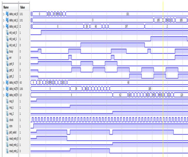
Fig.9 Router with Arbiter waveform
