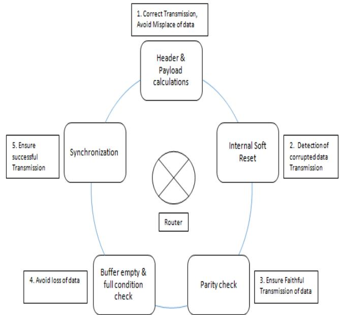
Fig.2 Fundamental Support by Router in NoC[5].
