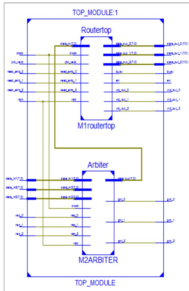
Fig.5 Top Level Architecture
