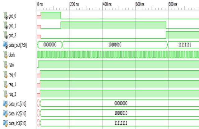
Fig.8 Arbiter waveform
