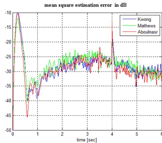
Fig. 5. The mean square estimation error (dB) of VLR algorithms.
