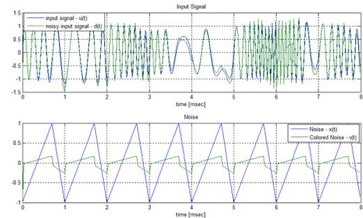
Fig. 6. Input signal, noisy input signal, and types of noise.
