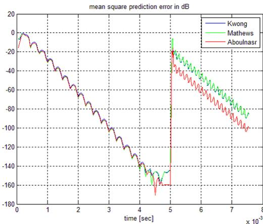
Fig. 3. The mean square prediction error of VLR algorithms for adaptive prediction.
