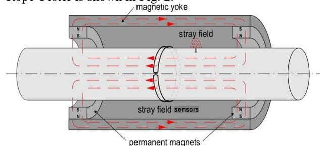
**Fig. 2. Schematic diagram of INTROS Rope Tester**
