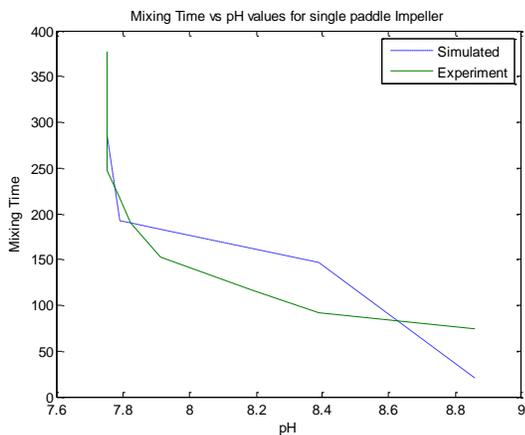
Fig. 4 Mixing Time Versus pH Value
