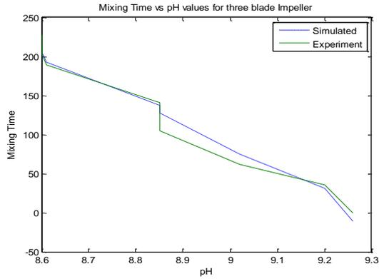
Fig. 2 Mixing Time Versus pH Value.
