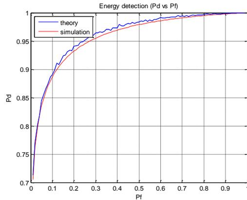
Fig 2: Detection probability vs false alarm probability of energy detector for 8PSK primary signal over AWGN channel in low SNR walls
