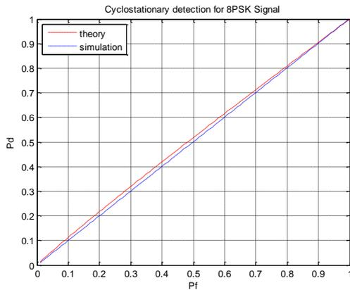
Fig 4: Detection probability vs false alarm probability of cyclostationary detector for 8PSK primary signal over AWGN channel in low SNR walls for SNR = -15dB
