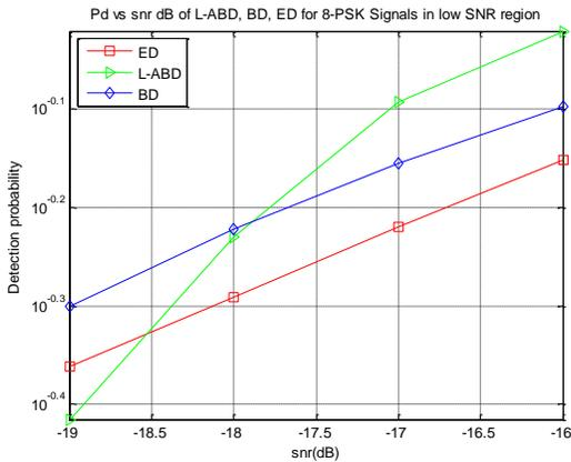
Fig 8: Detection probability vs SNR (dB) for 8PSK modulated primary user over AWGN channel in low SNR walls
