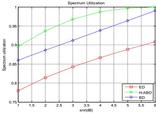
Fig 12: Spectrum utilization of 8PSK modulated primary signal over AWGN channel in High SNR walls
