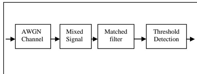
Fig 6: Principle of Matched filter operation
