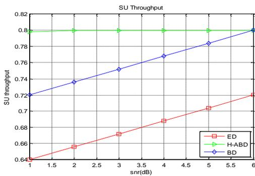
Fig 13: Secondary users' throughput of 8PSK modulated primary signal over AWGN channel in High SNR walls
