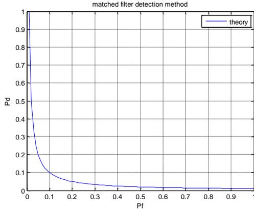
Fig 7: Theoretical detection probability vs false alarm probability of matched filter detector for 8PSK primary signal over AWGN channel in low SNR walls.
