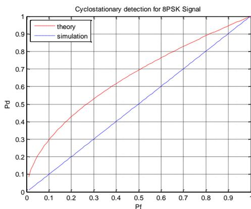
Fig 5: Detection probability vs false alarm probability of cyclostationary detector for 8PSK primary signal over AWGN channel in low SNR walls for SNR = -10dB
