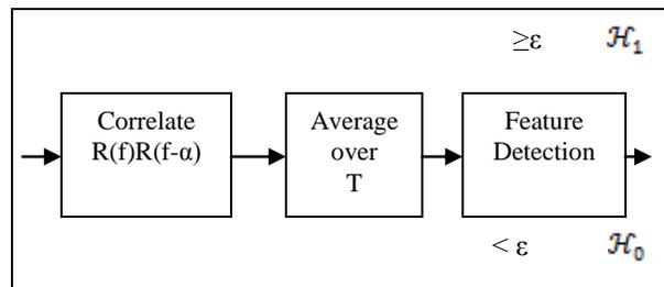
Fig 3: Principle of Cyclostationary method
