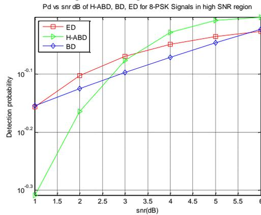
Fig 10: Detection probability vs SNR (dB) for 8PSK modulated primary user over AWGN channel in high SNR walls
