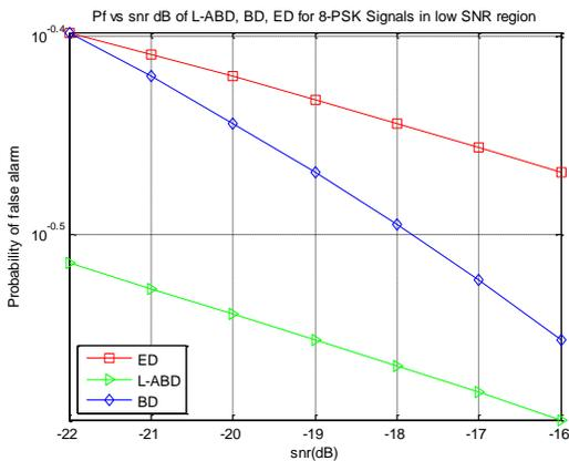
Fig 9: False alarm probability vs SNR (dB) for 8PSK modulated primary user over AWGN channel in low SNR walls
