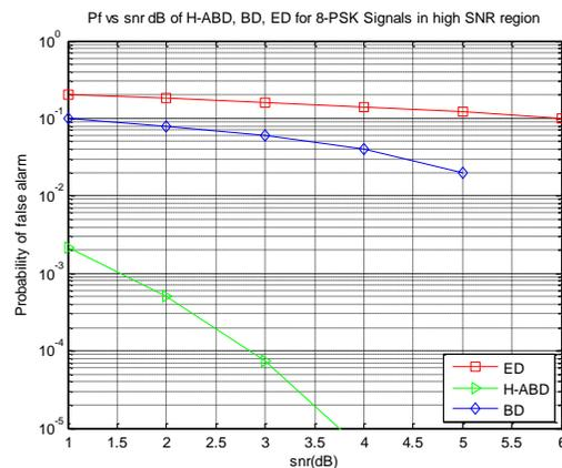
Fig 11: False alarm probability vs SNR (dB) for 8PSK modulated primary user over AWGN channel in high SNR walls
