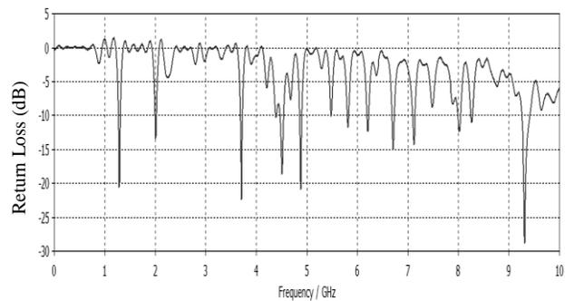
Fig. 5(b) Corresponding return loss vs frequency graph of Antenna-3.
