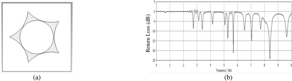
Fig. 8. (a) Antenna-6 with five triangular patches and curved edges.
