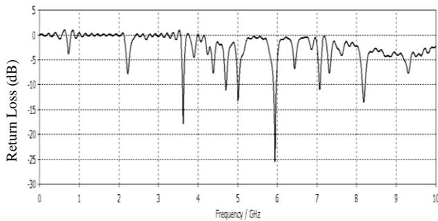
Fig. 2. Return loss vs frequency graph for Antenna-1.
