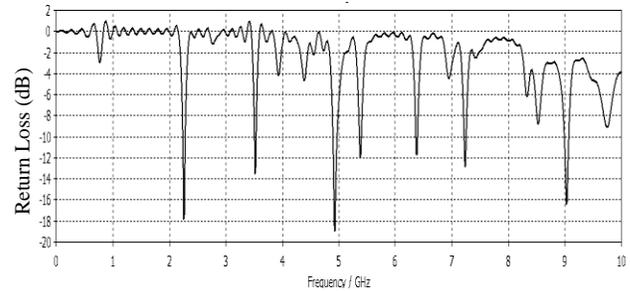
Fig. 4. Return loss vs frequency graph for Antenna-2.
