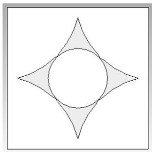
Fig. 3. Antenna-2 design with curved edges of the triangular patches.
