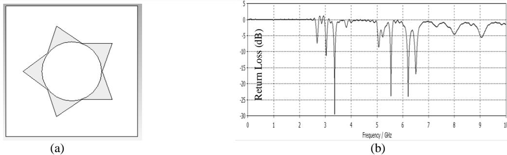
Fig. 7. (a) Antenna-5 with five triangular patches and straight edges.
