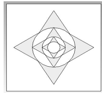
Fig. 5(a) Antenna-3 with straight edges and 3 fractal iterations
