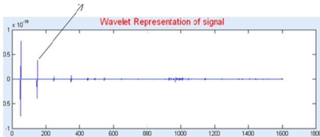
Figure -6-b. Wavelet representation of Faulty bearing
