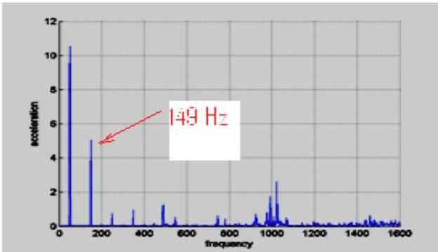
Table: 3 Frequency Vs Acceleration for faulty bearing
