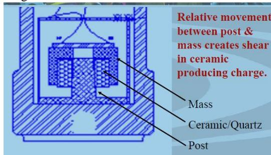
Figure: 2 Sectional view of Accelerometer
