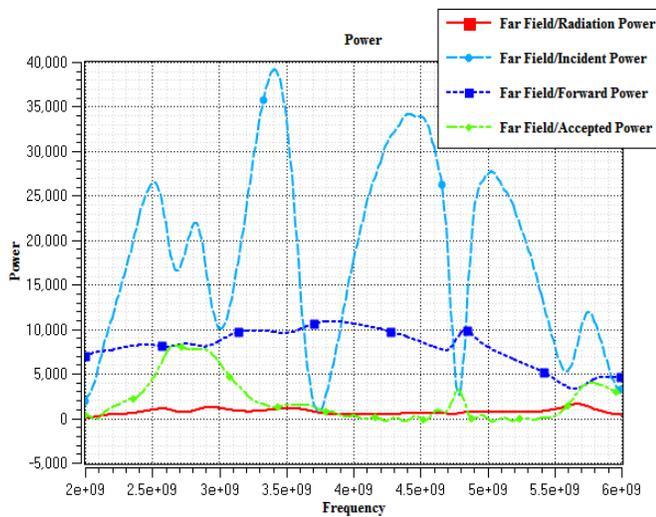
Fig.11: Power measurement of a connected E-shape & U-shape Microstrip patch antenna
