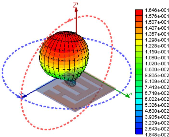
Fig.9: Gain at 2.66 GHz in 3D view with main design
