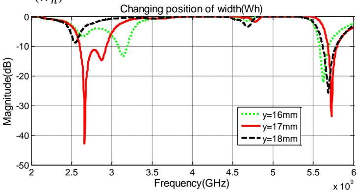
Fig.5: The variation of the position of the width (Wh) on the return loss response
