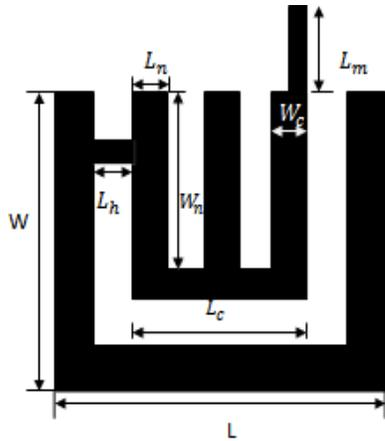
Fig.1: Structure of U-shape & E-shape Design
