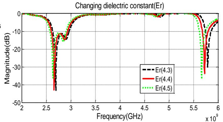
Fig.6: The variation of the of substrate dielectric constant (Er) on the return loss response
