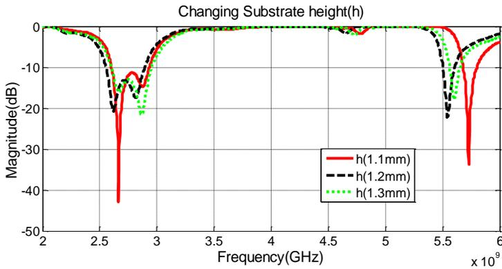
Fig.4: The variation of the of substrate height (h) on the return loss response
