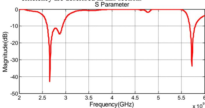
Fig.2: Return loss of Connected E-Shape & U-Shape Design
