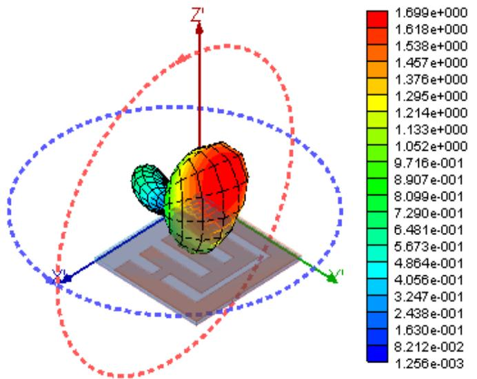
Fig.10: Gain at 5.72 GHz in 3D view with main design
