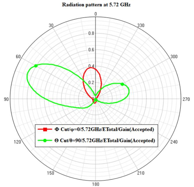
Fig.8: E-plane and H-plane at 5.72 GHz
