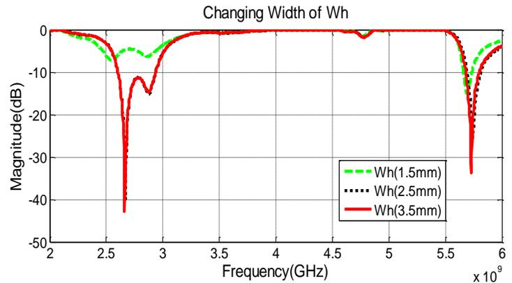
Fig.3: The variation of the ( $W_h$ ) parameter on the return loss response
