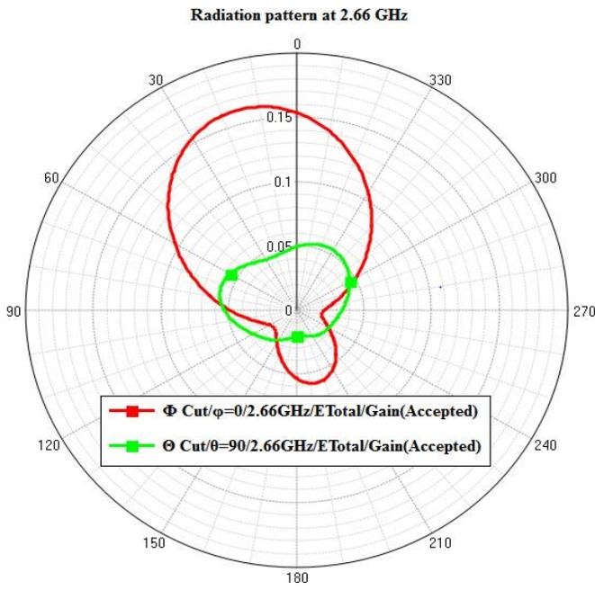
Fig.7: E-plane and H-plane at 2.66 GHz
