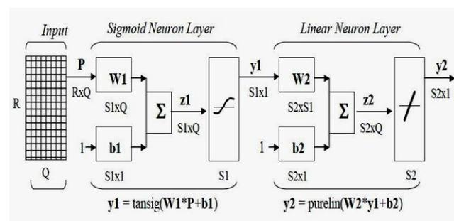
Fig. 1 A two layer feed forward neural network.
