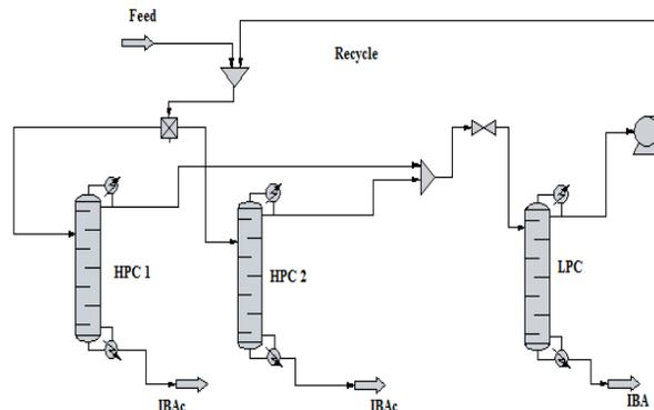
Figure 3. Three column process PSD for the separation of IBA-IBAc
