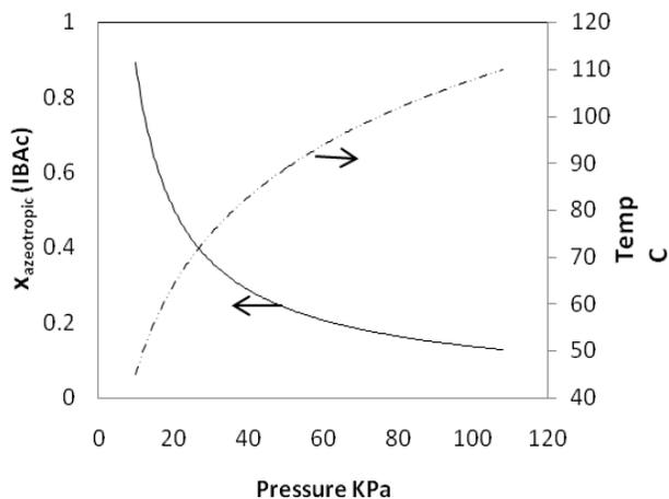
Figure 2. Azeotropic composition and temperature as function of Pressure
