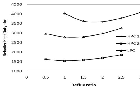
Figure 7. Variation in Reboiler duty with reflux ratio
