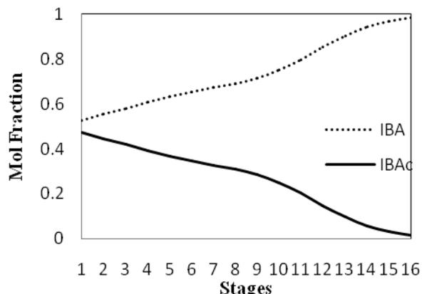
Figure 5. Liquid composition profile in HPC and LPC
