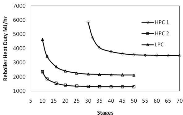
Figure 6. Variation of Reboiler duty with number of stages
