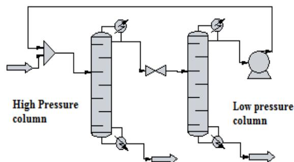
Figure 1. Conventional two column PSD process for separation for IBA-IBAc
