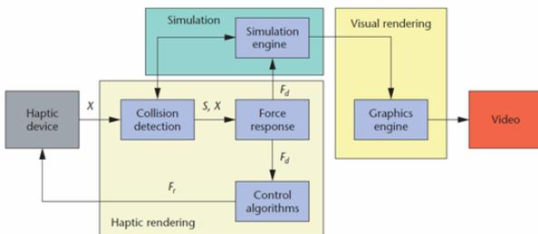
Fig. 2 Haptic System Diagram
