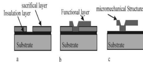
Fig. 2 Surface Micromachining
