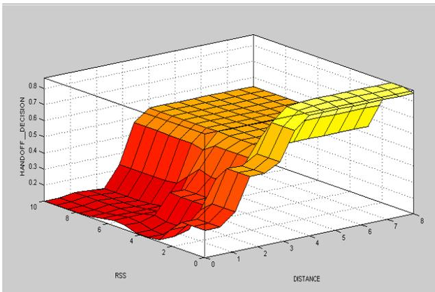
Figure 7. Surface curve between Distances, RSS & Handoff
