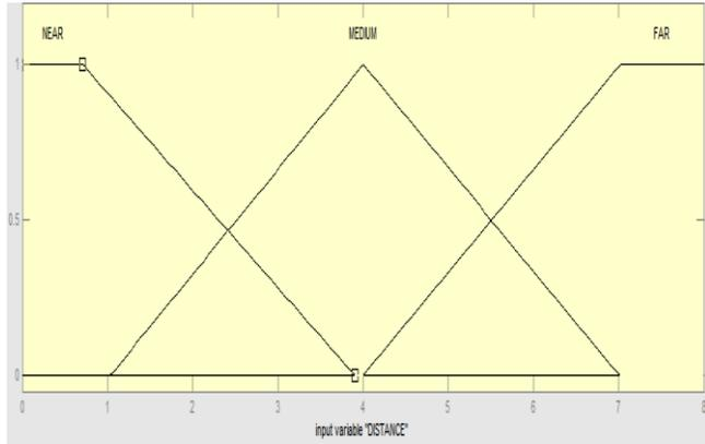
Figure 3. Membership functions of Distance between BS & MS
