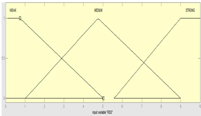
Figure 4. Membership functions of Received Signal Strength (RSS)
