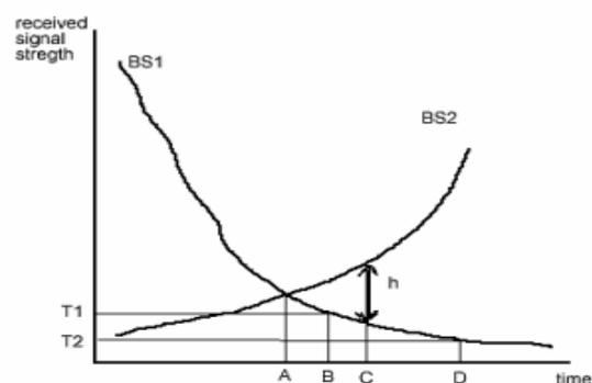
Figure 1. Conventional handoff based on RSS [3]
