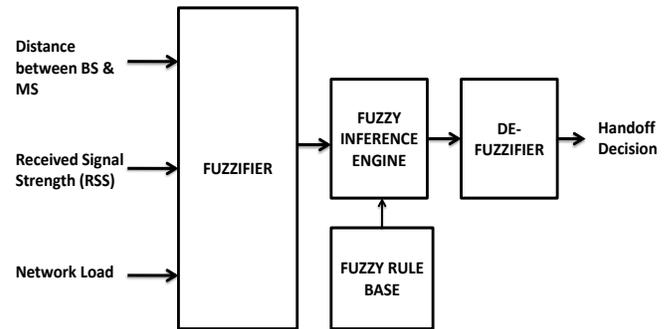
Figure 2. Block diagram Proposed fuzzy logic based handoff mechanism
