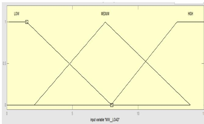
Figure 5. Membership functions of Network Load
