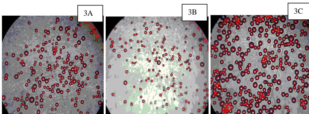
Figure 3.3. Extracted pore boundaries with active contour implementation.
