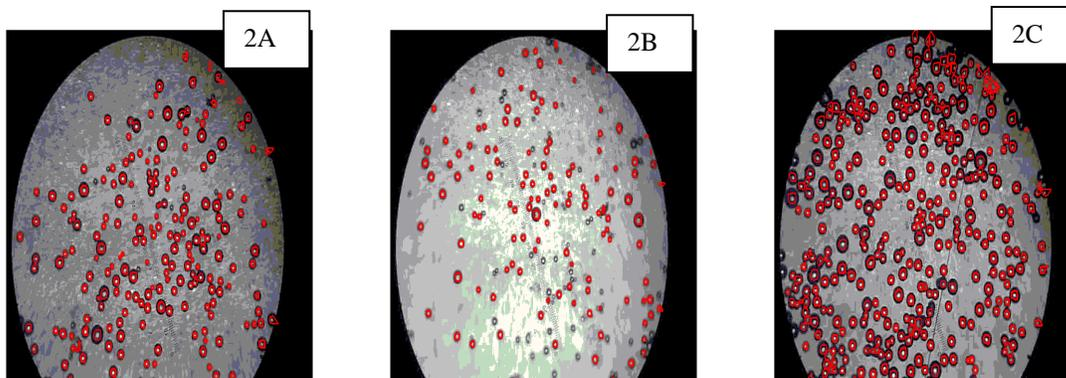
Figure 2.3. Extracted pore boundaries with watershed implementation.
