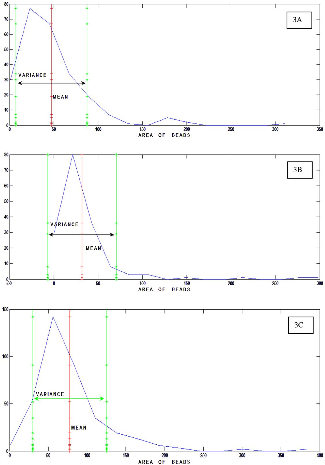
Figure 3.4. Area distribution of the three images with active contour method.
