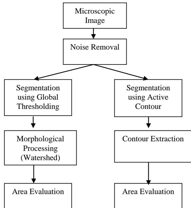
Figure 1. System model to compare the performance of active contour method with watershed technique.
